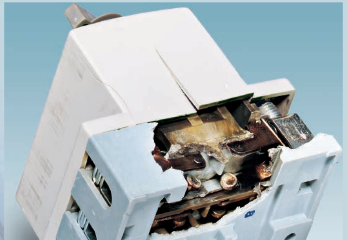
Fig. 1b: Destroyed residual current circuit breaker (RCD)
