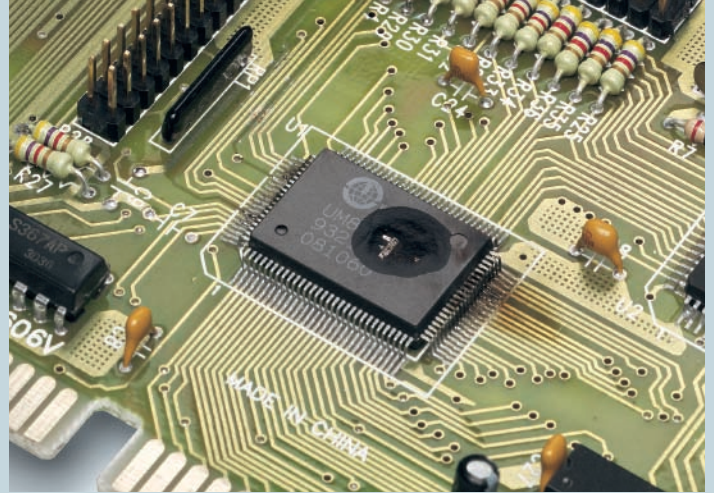
Fig. 1a: IC destroyed by surge voltages
